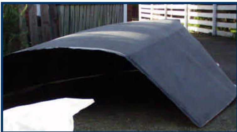
Photo 4 (above) shows the skin removed from the mould
