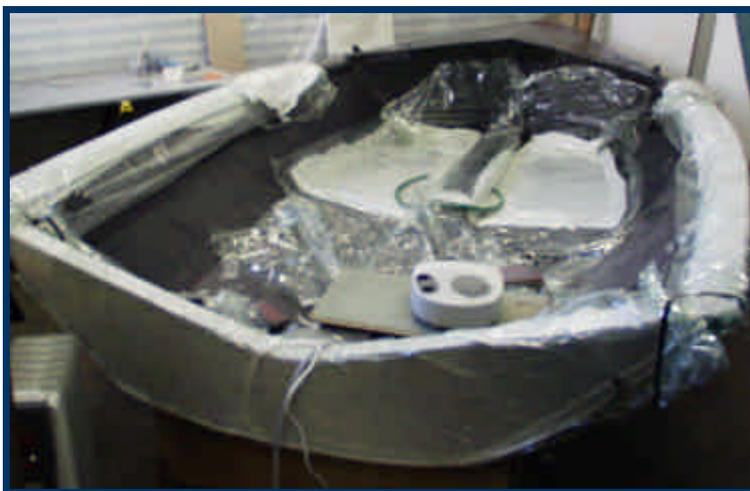
Photo 20 (above) the decks and transom being laminated and vacuum bagged
